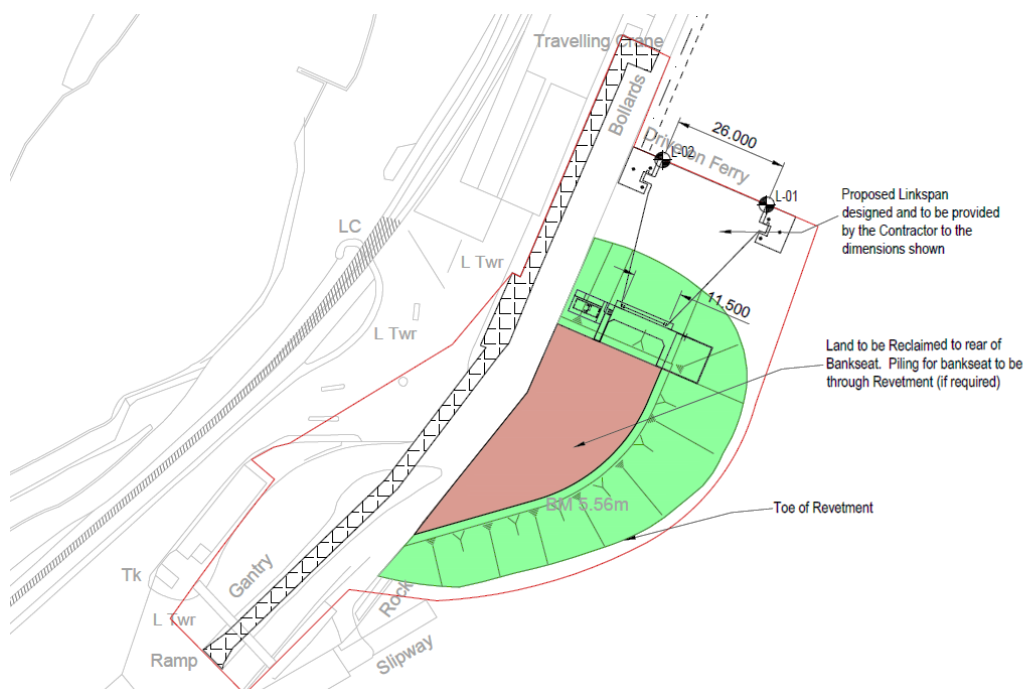
Figure 2.2: Proposed Layout of Replacement Linkspan (see also Volume II)
