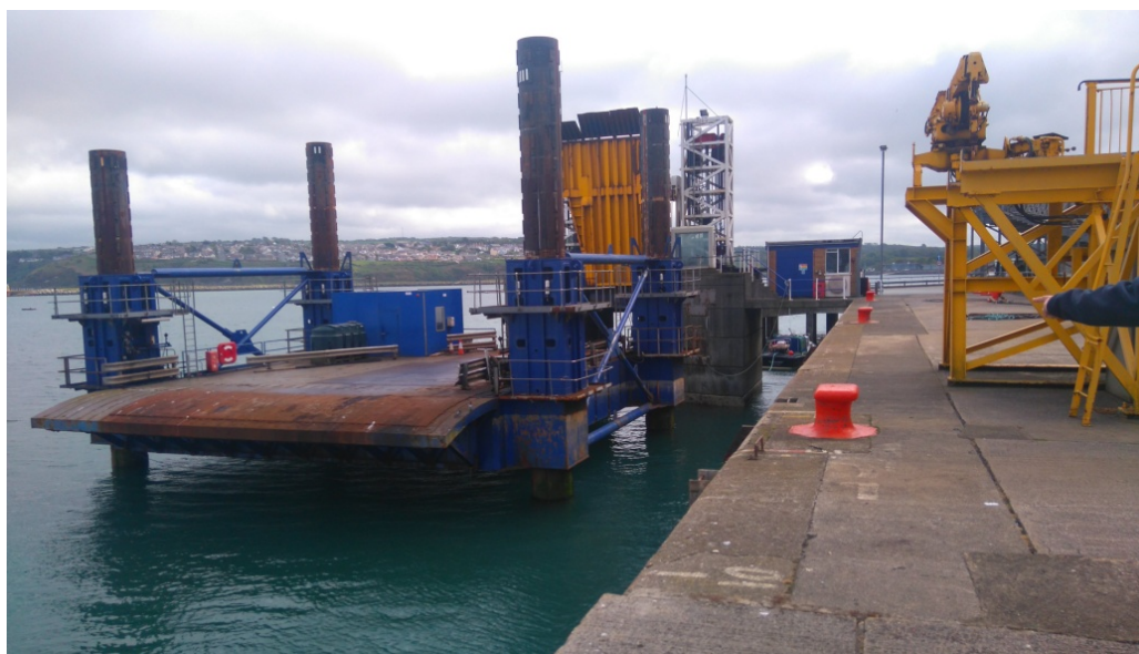
Figure 2.7 Existing Jack Up Structure and piles
