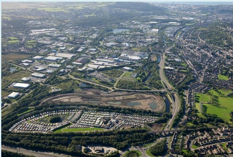
**Figure 13: Aerial view of site during construction in September 2013 looking south. The new set-back flood embankment is now operational as the old embankment is being removed. Landscaping of the wetland habitat is under construction.**
