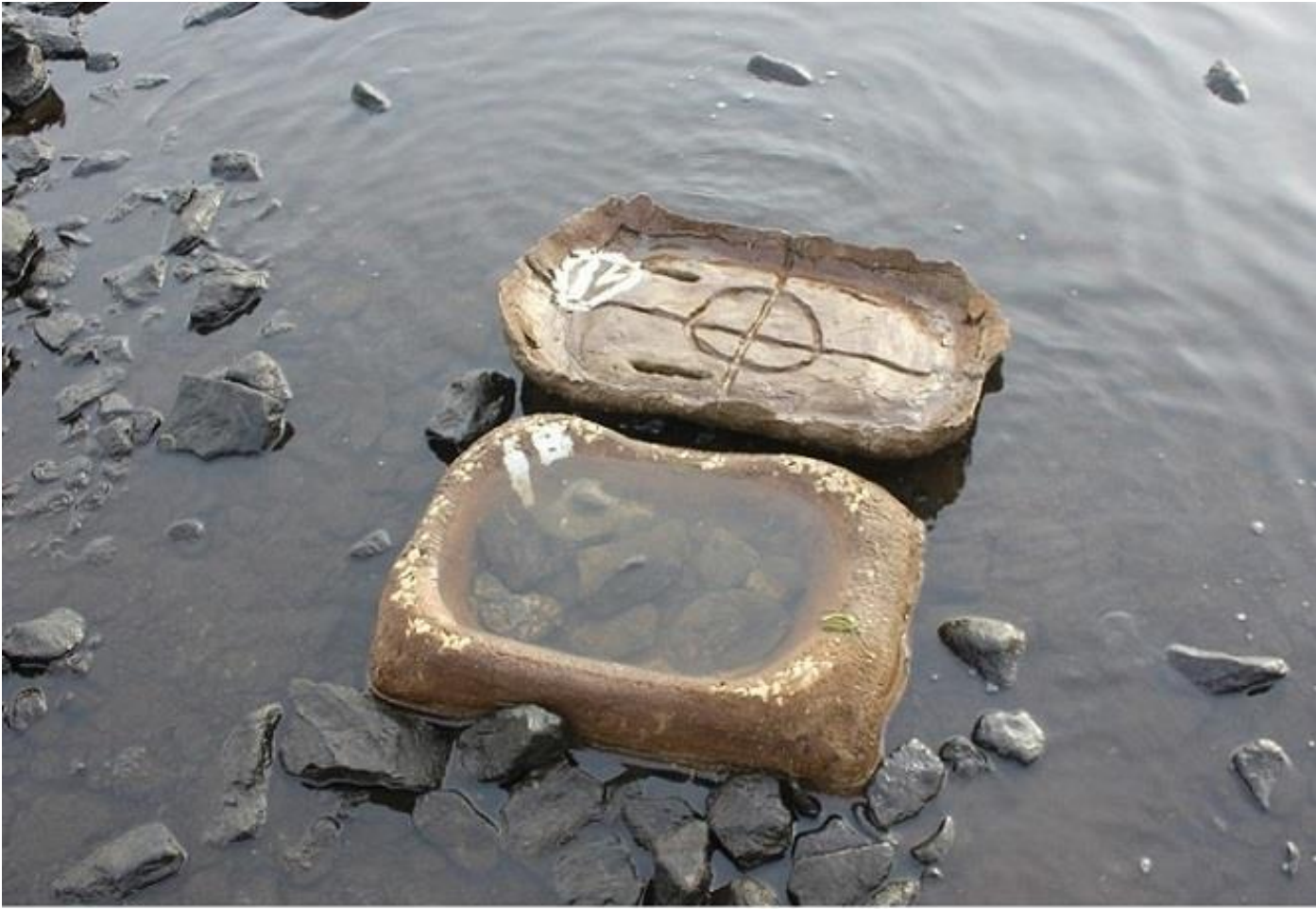
The open refuge at the shallowest point at Site 1 North Pier just over one month after installation (in 500mm deep water)
