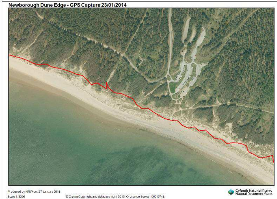
Figure 28. Retreat of frontal dunes at Newborough Warren after the winter storms. Red line indicates current line of frontal dunes compared to the situation in 2009.
