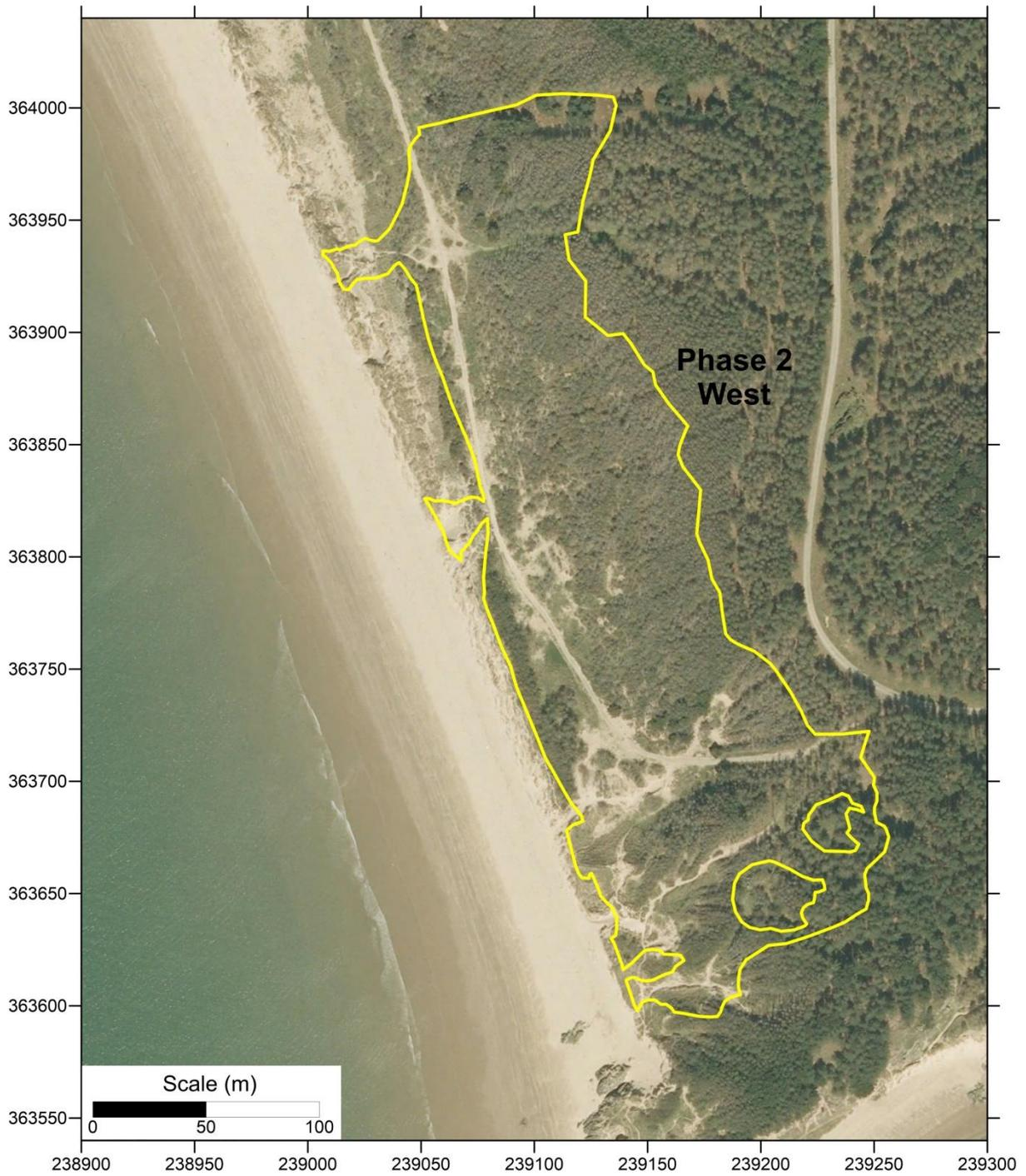
**Figure 61.** Pre-works aerial photograph flown 11 May 2009 of the Phase 2 West rejuvenation trial area (at Traeth Penrhos). The yellow lines indicate the bare sand (vegetation stripping and sand heaps) created in December 2014 to March 2015, as surveyed on 25-27 March 2015 by ground RTK-GPS survey
