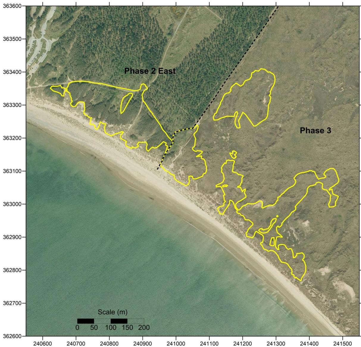
**Figure 71.** Pre-works aerial photograph flown 11 May 2009, showing boundaries of the Newborough Phase 2 East and Phase 3 rejuvenation trial areas (separated with the dashed black line). The yellow lines indicate the bare sand (vegetation stripping and sand ridges and heaps) created in December 2014 to March 2015, as surveyed on 25-27 March 2015 by ground RTK-GPS survey
