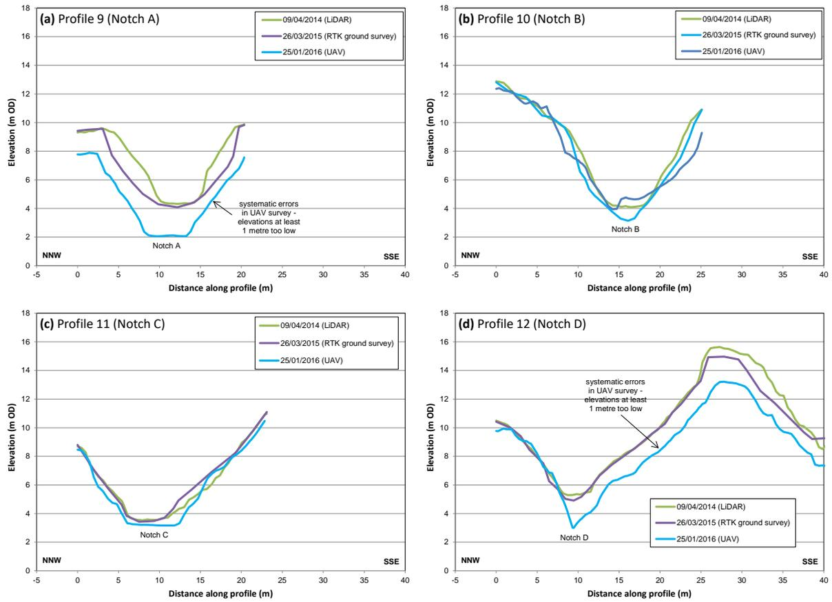
**Figure 70.** Topographic profiles across notches in the Phase 2 West area of Newborough (at Traeth Penrhos). Post-works elevations are shown for the aerial LiDAR survey flown 09/04/2014, the subsequent ground RTK survey on 26/03/2015, and UAV survey on 25/01/2016. Note that the 2016 UAV survey data are at least 1 metre too low on Profiles 9 and 12 due to a greater distance from the control points which were located in the centre of the site
