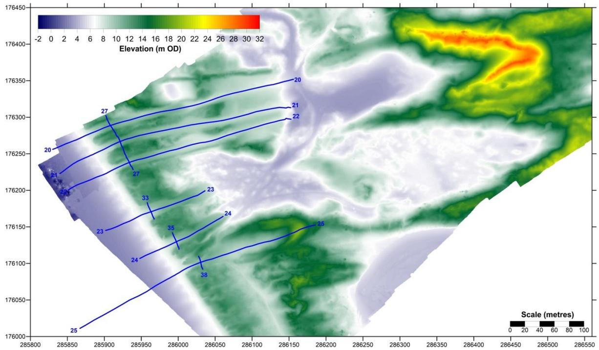
**Figure 43.** DEM of Merthyr Mawr Warren based on the UAV survey on 29 February 2016, after correction to ODN
