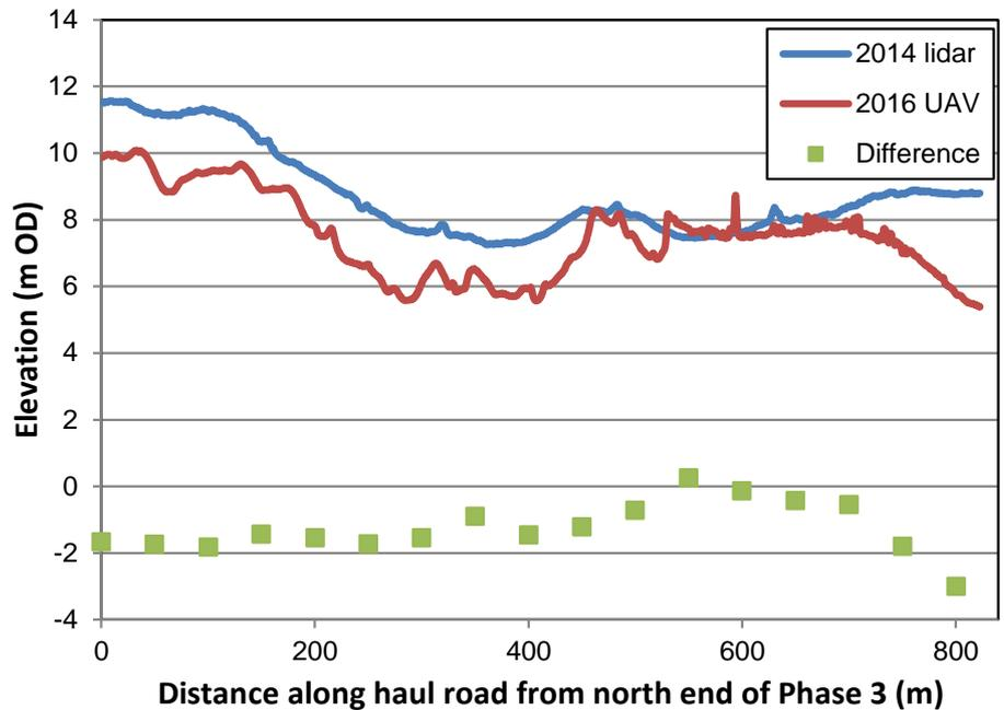
**Figure 17.** Comparison of elevation units measured during 2014 LiDAR survey and 2016 UAV survey, after translation of 3 m to the south and 5 m to the west, and conversion to m ODN using the addition of +17.0 m. The differences along the haul road were extrapolated in a WSW-ENE direction, and the DEM warped in Surfer
