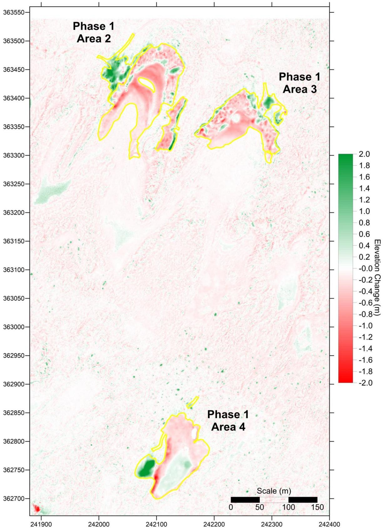
**Figure 55.** Difference in elevation between May 2009 and April 2014 aerial LiDAR surveys. Total volume changes before and after the works are negligible and within the error limits of the two surveys. The slight apparent increase in elevation within the southern part of Area 4 is due to presence of standing water
