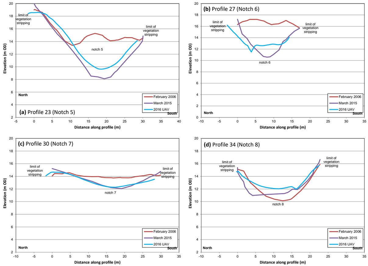
**Figure 24.** Topographic profiles across the notches in the Kenfig Phase 3 area. Elevations are shown for the aerial LiDAR survey flown prior to rejuvenation works (26 February 2006), subsequent ground RTK surveys in May 2013, March 2014 and March 2015, and UAV survey on 2 March 2016 (note that although corrections have been made, the data are still unreliable, most notable for Notch 4)
