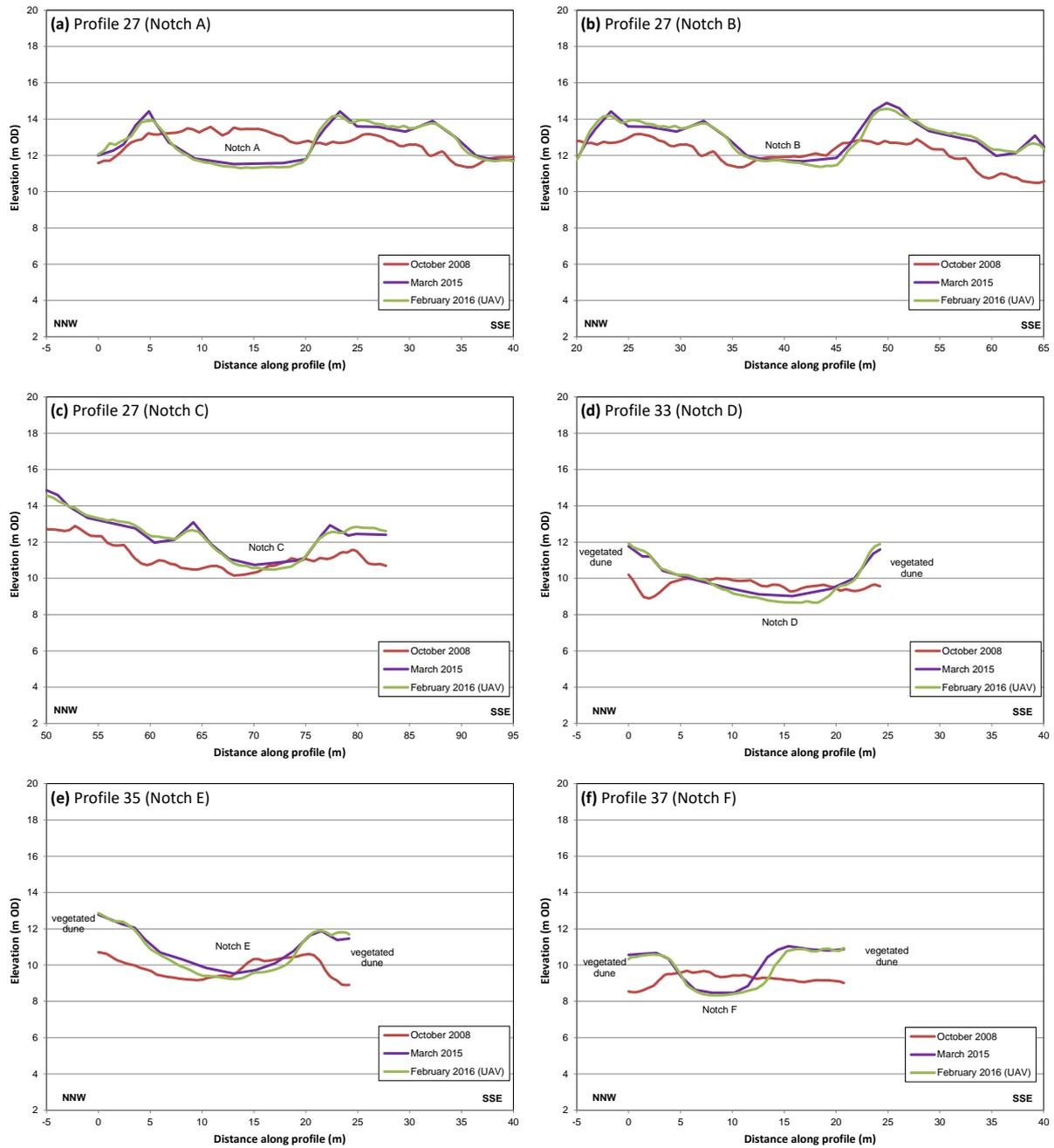
**Figure 47.** Topographic profiles across notches in the Phase 3 area at Merthyr Mawr Warren. Elevations are shown for the aerial LiDAR survey flown prior to rejuvenation works (October 2008), the subsequent ground RTK survey in March 2015 and aerial drone survey in March 2016
