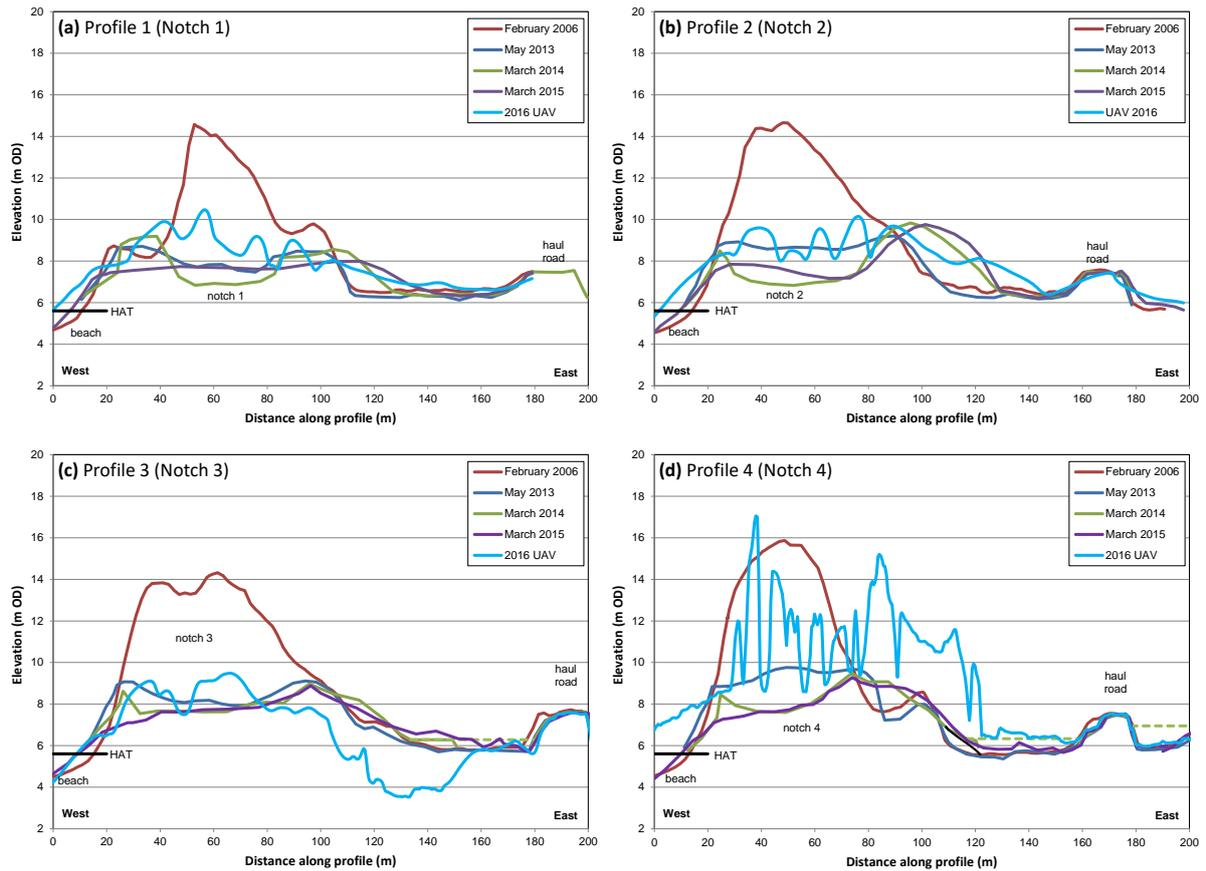
**Figure 21.** Topographic profiles along the axes of the notches in the Kenfig Phase 2 area. Elevations are shown for the aerial LiDAR survey flown prior to rejuvenation works (26 February 2006), subsequent ground RTK surveys in May 2013, March 2014 and March 2015, and UAV survey on 2 March 2016 (note that although corrections have been made, the data are still some unreliable). The level of HAT (at 5.6 m ODN) is also shown
