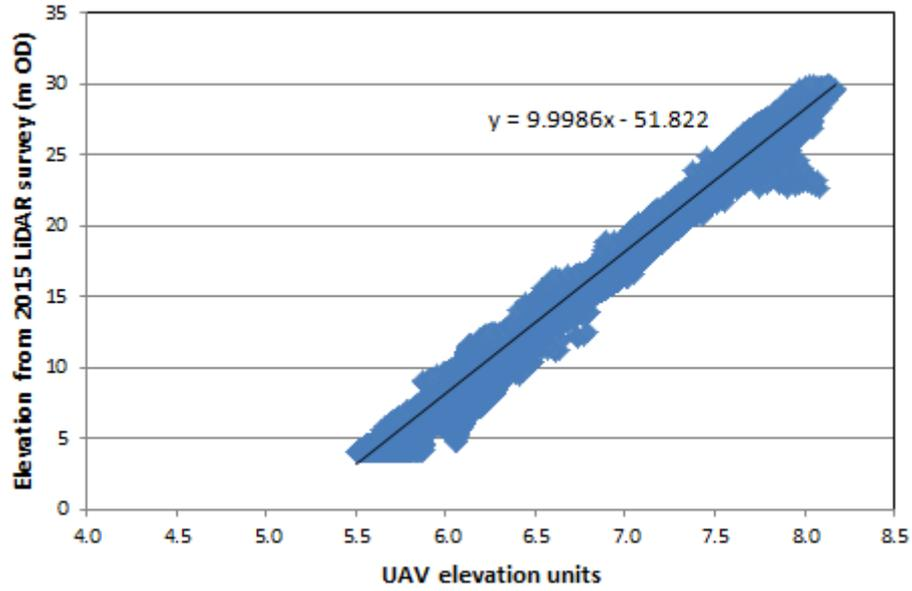
**Figure 42.** Comparison of elevation units measured during 2014 LiDAR survey and 2016 UAV survey. A linear trend line shows the correction required to adjust elevation units to ODN
