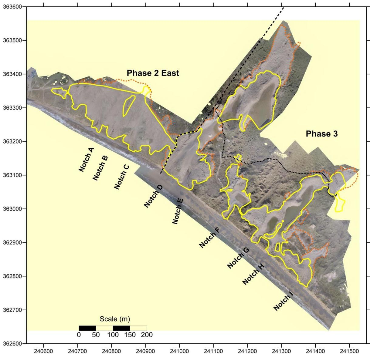
**Figure 72.** UAV aerial imagery flown January 2016 showing the extent of bare sand on the Phase 2 East and Phase 3 rejuvenation works at Newborough, undertaken December 2014 to March 2015. The yellow lines indicate the bare sand areas created in December 2014 to March 2015, the orange dashed lines the areas of blown sand outside the works areas by January 2016 (note that some areas are estimated due to incomplete UAV coverage)
