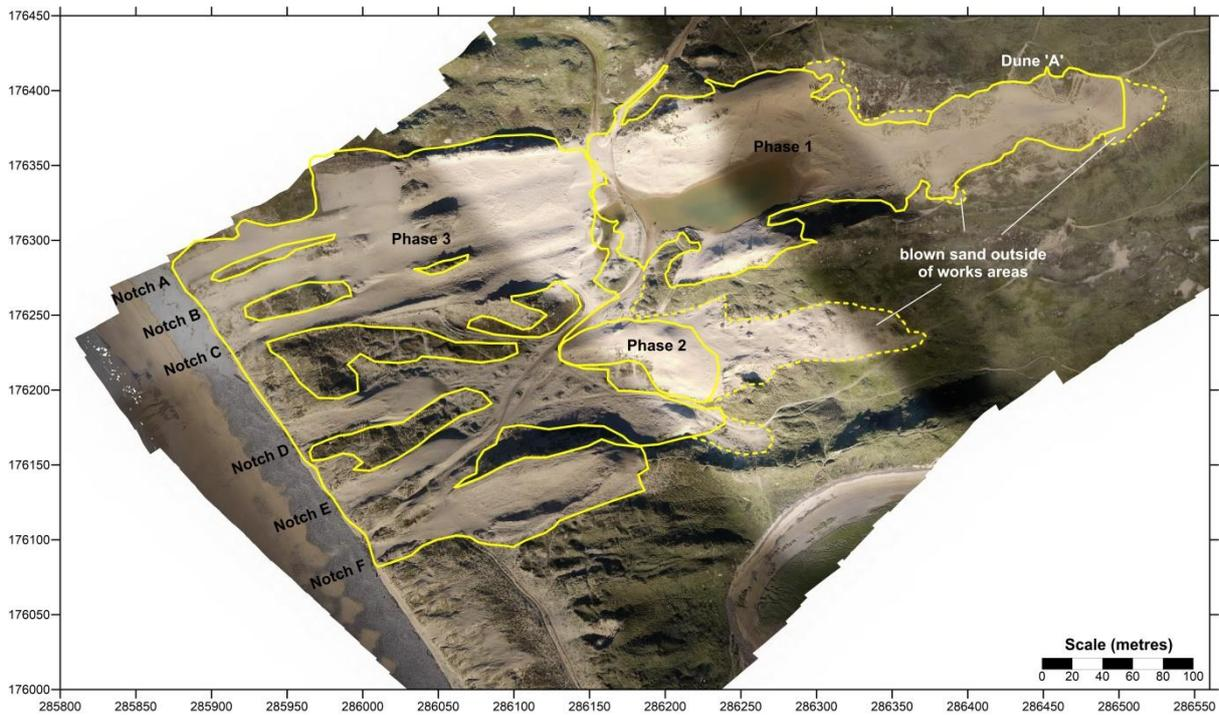
**Figure 38.** Composite aerial photograph mosaic of the dune rejuvenation area at Merthyr Mawr based on UAV survey 29 February 2016, showing the three phases of dune rejuvenation works
