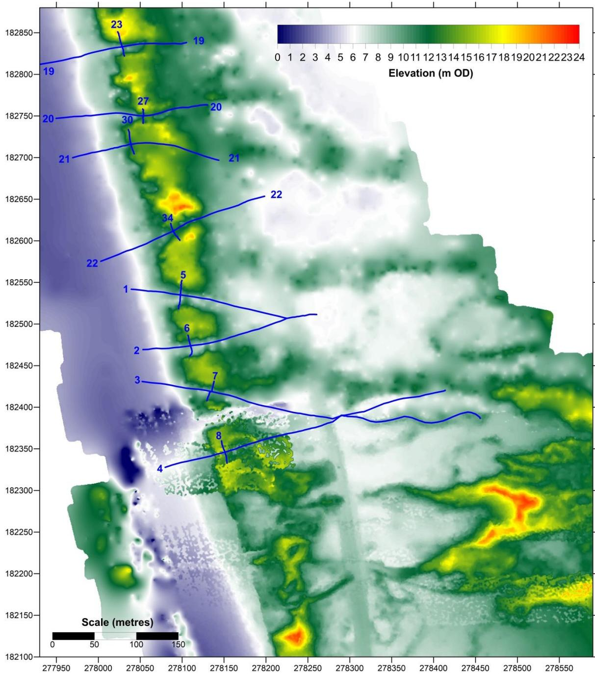
**Figure 18.** DEM of the Kenfig site based on the UAV survey flown on 02 March 2016, after correction using the elevations recorded along the haul road on the 2014 LiDAR survey
