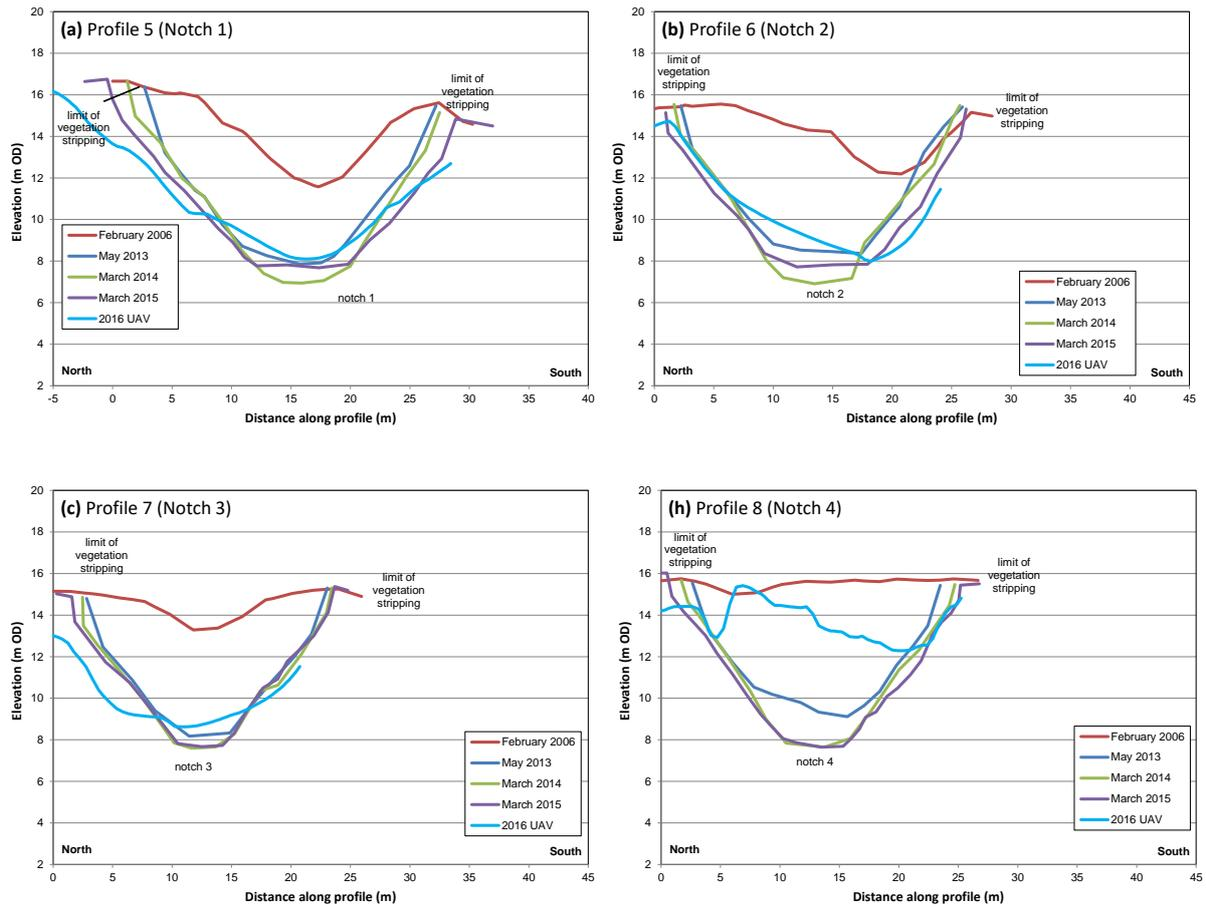
**Figure 22.** Topographic profiles across the notches in the Kenfig Phase 2 area. Elevations are shown for the aerial LiDAR survey flown prior to rejuvenation works (26 February 2006), subsequent ground RTK surveys in May 2013, March 2014 and March 2015, and UAV survey on 2 March 2016 (note that although corrections have been made, the data are still unreliable, most notably for Notch 4)
