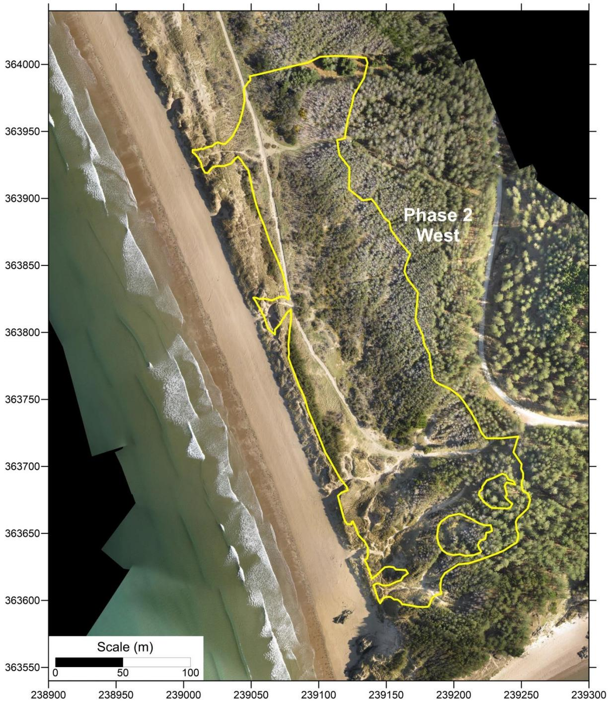
**Figure 62.** Pre-works aerial photograph flown June 2013 by UAV of the Phase 2 West rejuvenation trial area (at Traeth Penrhos). The yellow lines indicate the bare sand (vegetation stripping and sand heaps) created in December 2014 to March 2015, as surveyed on 25-27 March 2015 by ground RTK-GPS survey
