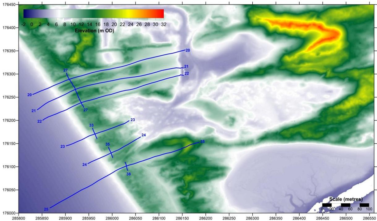
**Figure 40.** Unfiltered DEM of Merthyr Mawr Warren based on an aerial LiDAR survey on 5 February 2015, after all the rejuvenation works Phases 1-3
