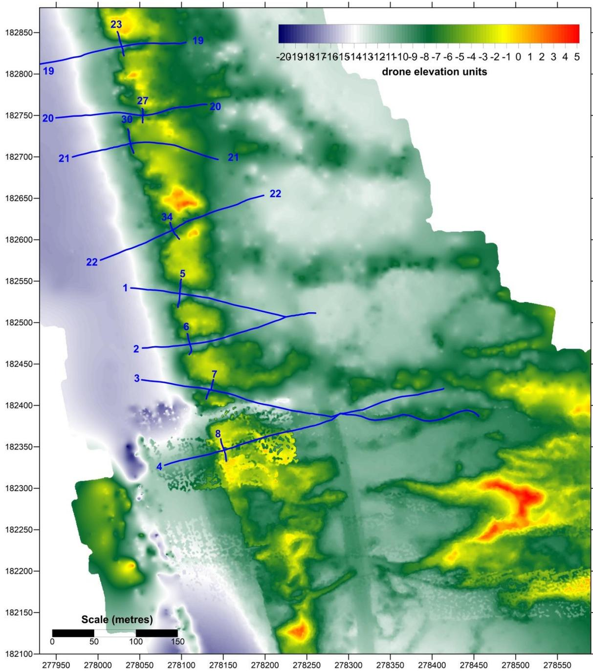
**Figure 15.** Unfiltered DEM of the Kenfig site based on the UAV survey on 02 March 2016. Data are shown as supplied, without correction to ODN. Note the elevation scale ranges from -20 to + 5
