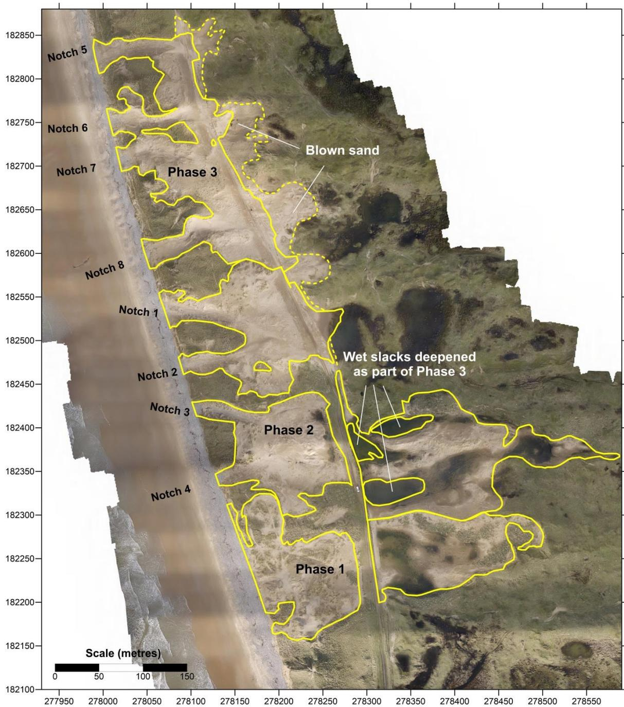
**Figure 12.** UAV aerial imagery flown February 2016 showing the extent of bare sand associated with the three phases of dune rejuvenation works at Kenfig undertaken February to March 2012 (Phase 1), January to February 2013 (Phase 2) and November to December 2014 (Phase 3)
