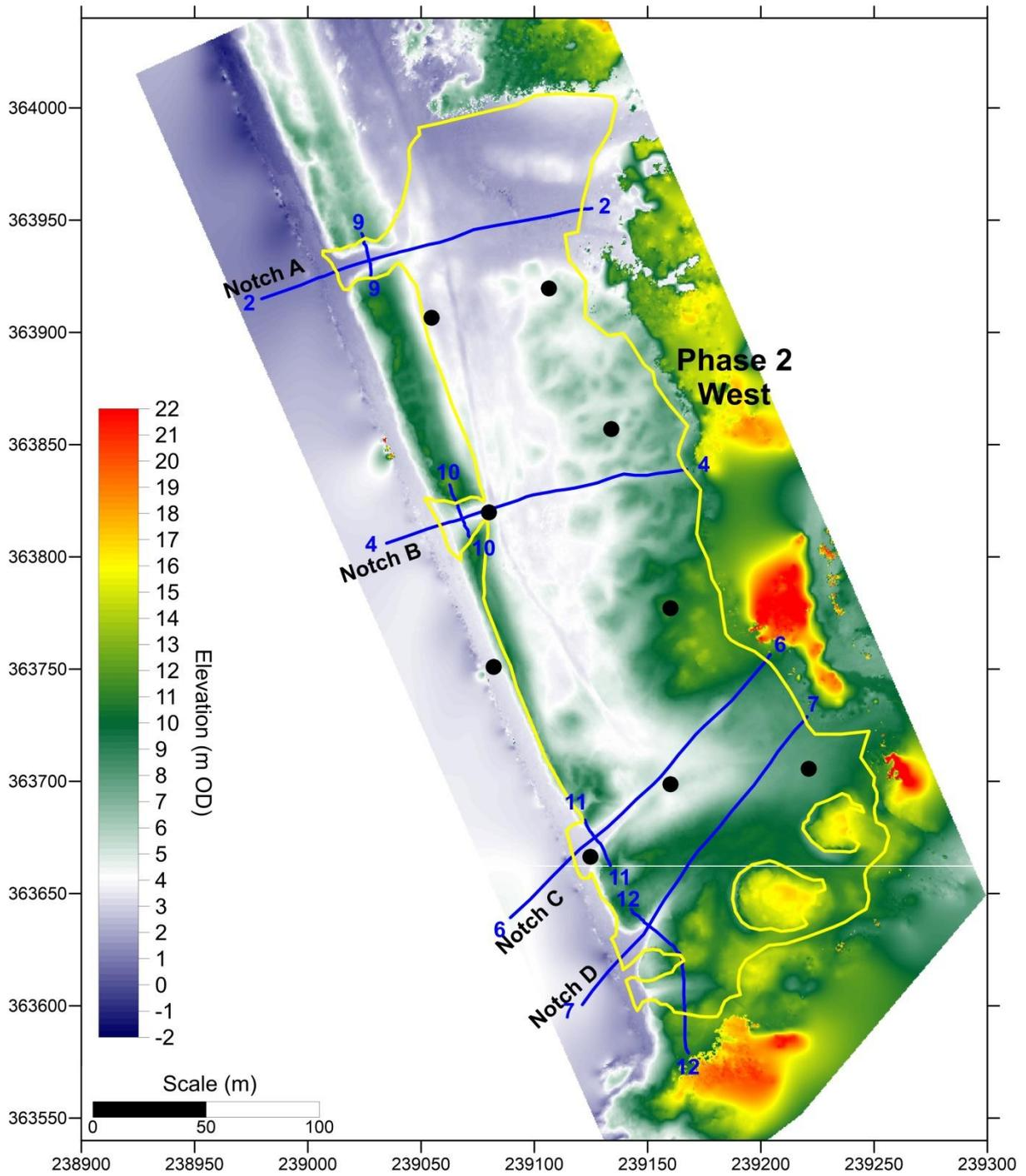
**Figure 67.** DEM of Newborough Phase 2 West area, from a UAV survey flown in January 2016, after the rejuvenation works. The calibration points used by the survey company to correct the elevations are shown as black dots
