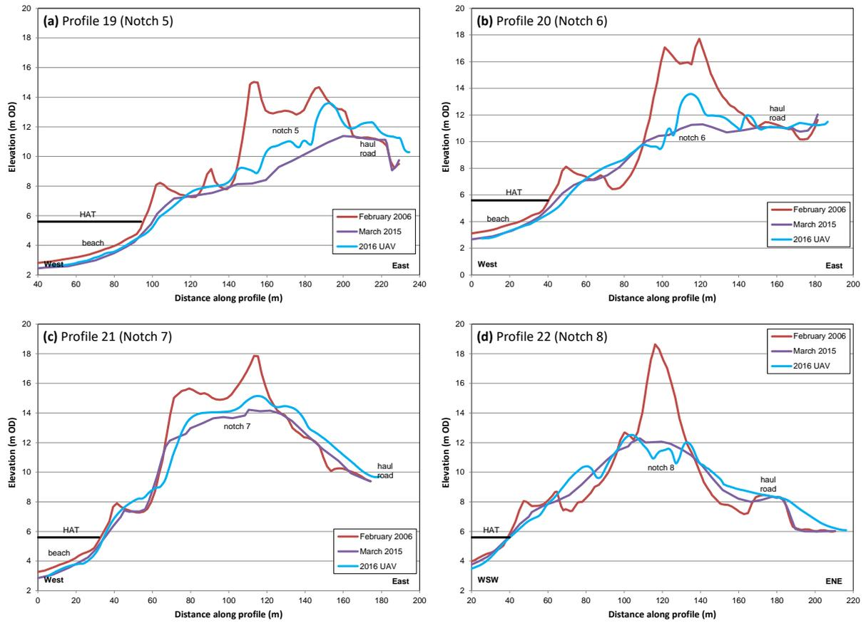
**Figure 23.** Topographic profiles along the axes of the notches in the Kenfig Phase 3 area. Elevations are shown for the aerial LiDAR survey flown prior to rejuvenation works (26 February 2006), subsequent ground RTK surveys in May 2013, March 2014 and March 2015, and UAV survey on 2 March 2016 (note that although corrections have been made, the data are unreliable). The level of HAT (at 5.6 m ODN) is also shown
