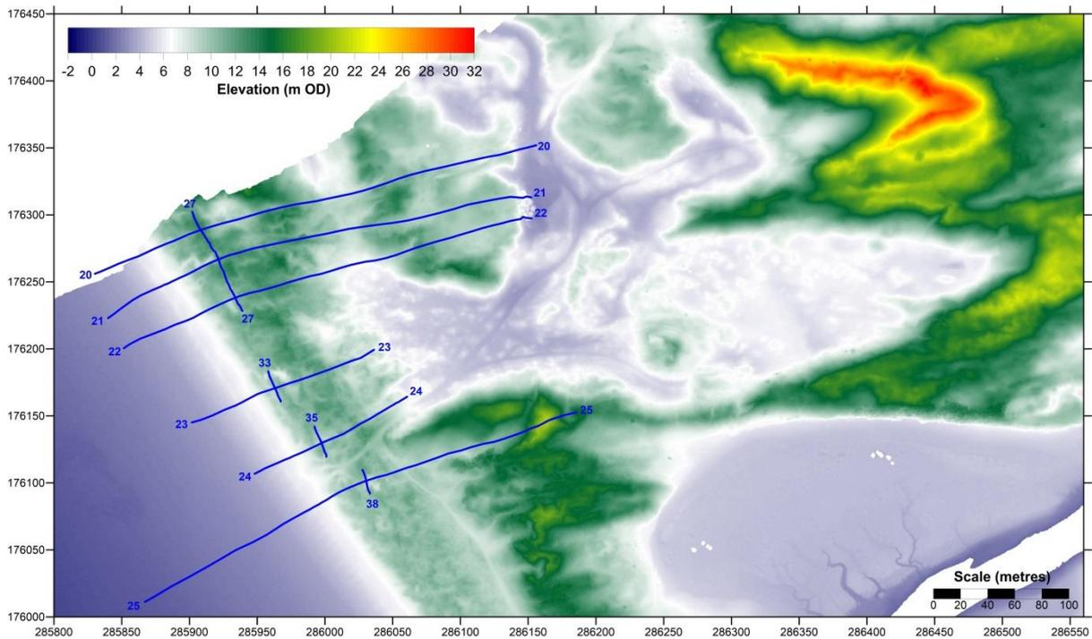
**Figure 39.** Unfiltered DEM of Merthyr Mawr Warren based on an aerial LiDAR survey on 16-29 October 2008, before rejuvenation works
