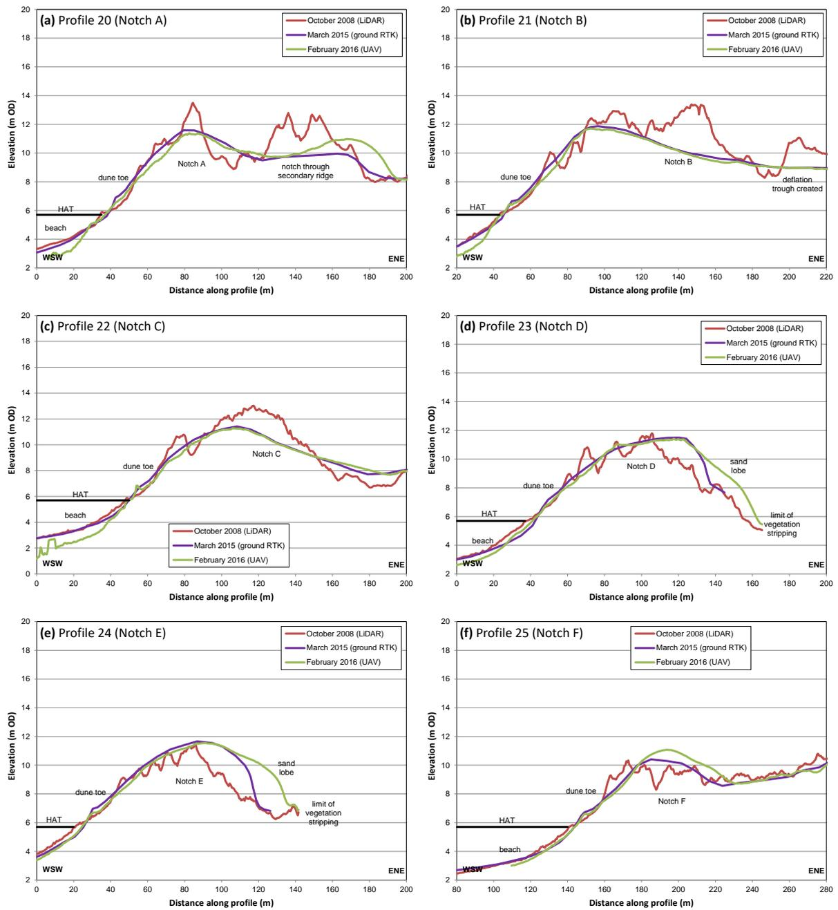
**Figure 46.** Topographic profiles along the axes of the notches in the Phase 3 area at Merthyr Mawr Warren. Elevations are shown for the aerial LiDAR survey flown prior to rejuvenation works (October 2008), the subsequent ground RTK survey in March 2015 and UAV survey in March 2016. The level of HAT (at 5.7 m ODN) is also shown
