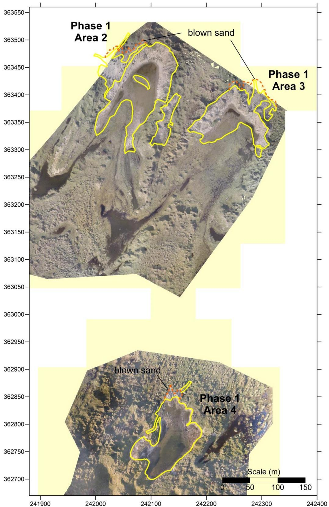
**Figure 52.** UAV aerial imagery flown January 2016 showing the extent of bare sand on the Phase 1 rejuvenation works at Newborough Warren, undertaken February to April 2013. The yellow lines indicate the areas to be stripped in February to April 2013, the orange dashed lines the areas of blown sand outside the works areas by January 2016 (note that some areas are estimated due to incomplete UAV coverage)
