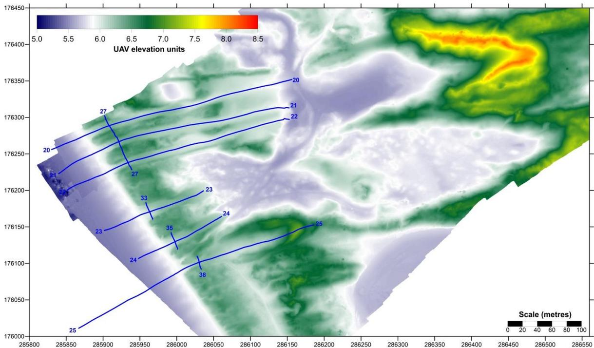
**Figure 41.** Unfiltered DEM of Merthyr Mawr Warren based on the UAV survey on 29 February 2016. Data are shown as supplied, without correction to ODN. Note the elevation scale ranges from 5.0 to 8.0 units
