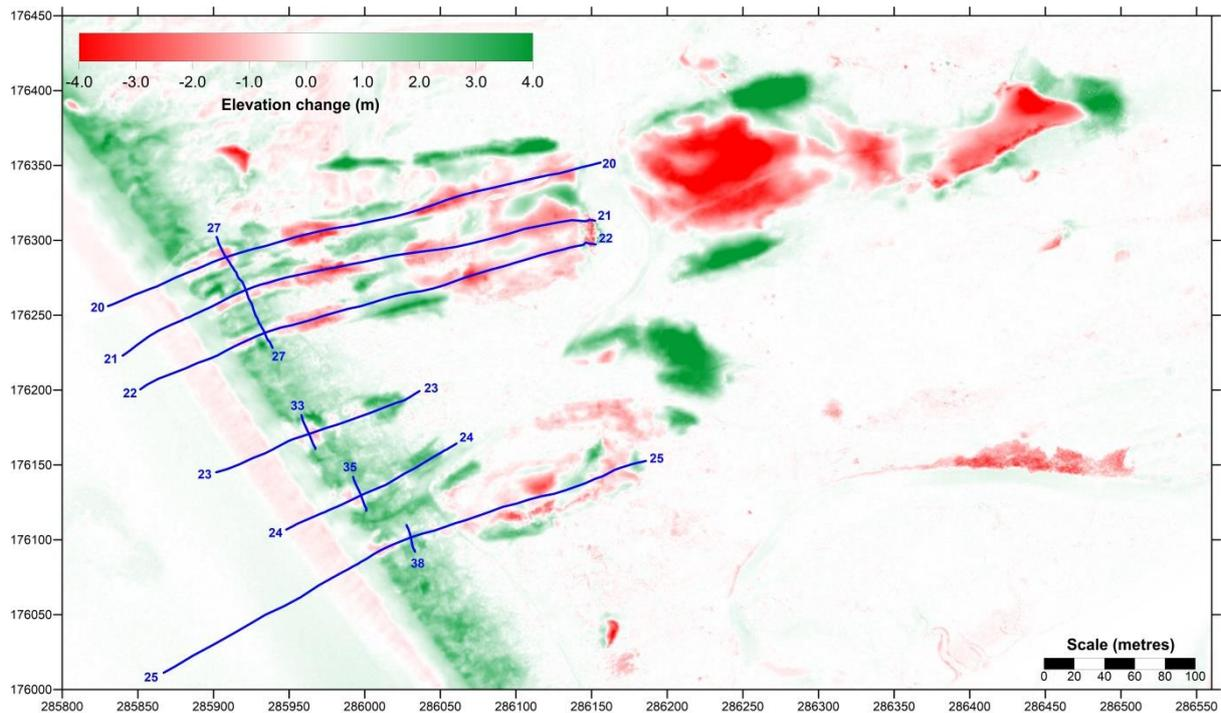
**Figure 44.** Difference in elevation between 2008 and 2015 aerial LiDAR surveys. Across the Phase 1-3 areas, and above the HAT contour in 2008, there was approximately 54000 m<sup>3</sup> of sediment accretion and 38751 m<sup>3</sup> of erosion, equating to a net sediment volume increase of approximately 15330 m<sup>3</sup> arising from new sediment input from the beach
