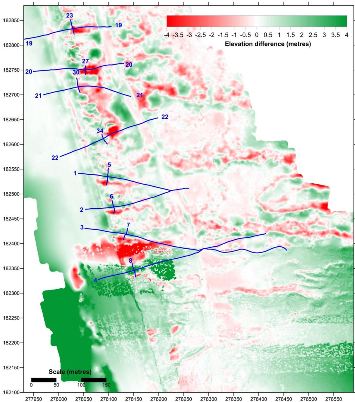
**Figure 20.** Difference in apparent elevation between the Kenfig 2014 aerial LiDAR and 2016 UAV survey, after corrections using the elevations recorded along the haul road on the 2014 LiDAR survey. Note that the apparent elevations in the southern third of the image are unreliable
