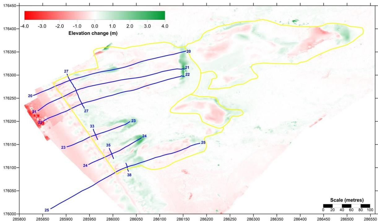
**Figure 45.** Difference in elevation between 2015 aerial LiDAR and 2016 UAV surveys. Across the Phase 1-3 areas, and above the HAT contour in 2008, there was approximately 13770 m<sup>3</sup> of sediment accretion and approximately 8100 m<sup>3</sup> of sediment erosion, equating to a net volume increase of approximately 5670 m<sup>3</sup> due to input of new sediment from the beach
