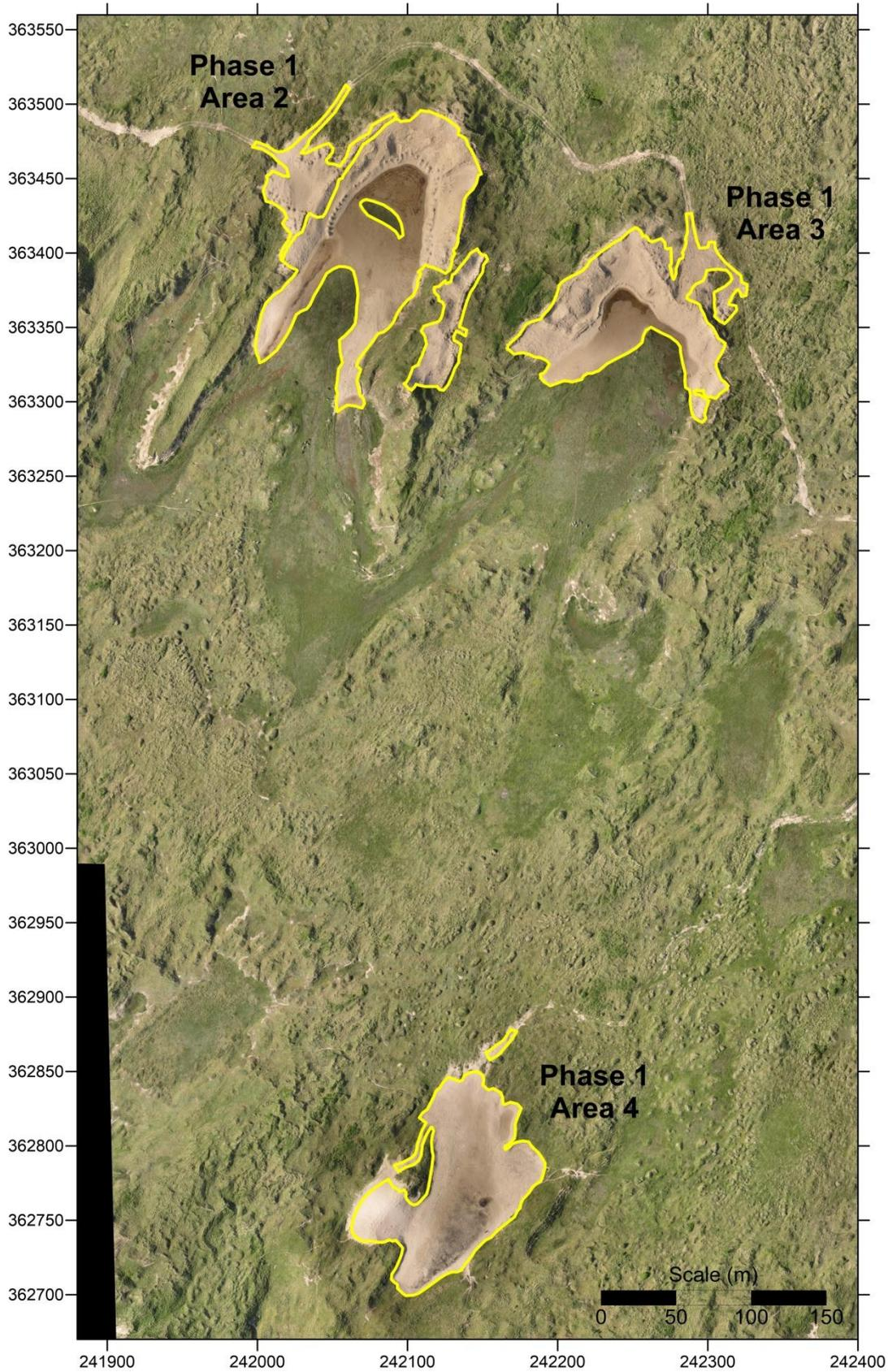
**Figure 51.** Aerial photograph flown June 2013 by UAV, showing extent of bare sand on the Phase 1 rejuvenation trial areas. The yellow lines indicate the areas to be stripped in February to April 2013, as surveyed on 16-17 May 2013 by ground RTK-GPS survey
