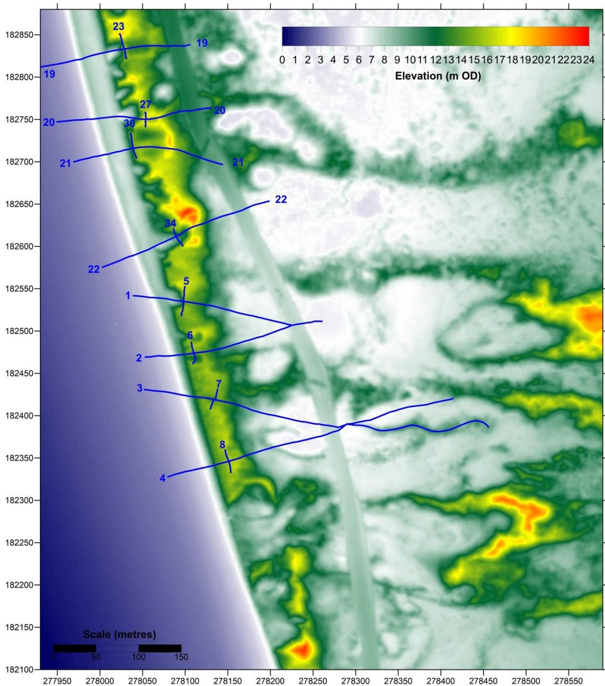
**Figure 13.** Unfiltered DEM of the Kenfig rejuvenation site, based on an aerial LiDAR survey on 26 February 2006, before the rejuvenation works started
