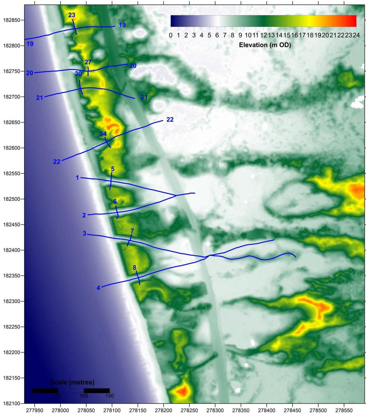
**Figure 14.** Unfiltered DEM of the Kenfig rejuvenation site based on an aerial LiDAR survey on 31 March 2014, after completion of the Phase 1 and Phase 2 works but before the Phase 3 works
