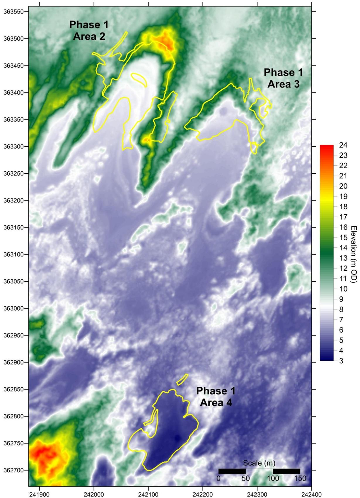
**Figure 53.** Filtered DEM of Newborough Warren Phase 1 areas, from an aerial LiDAR survey flown on 12 May 2009, before the rejuvenation works
