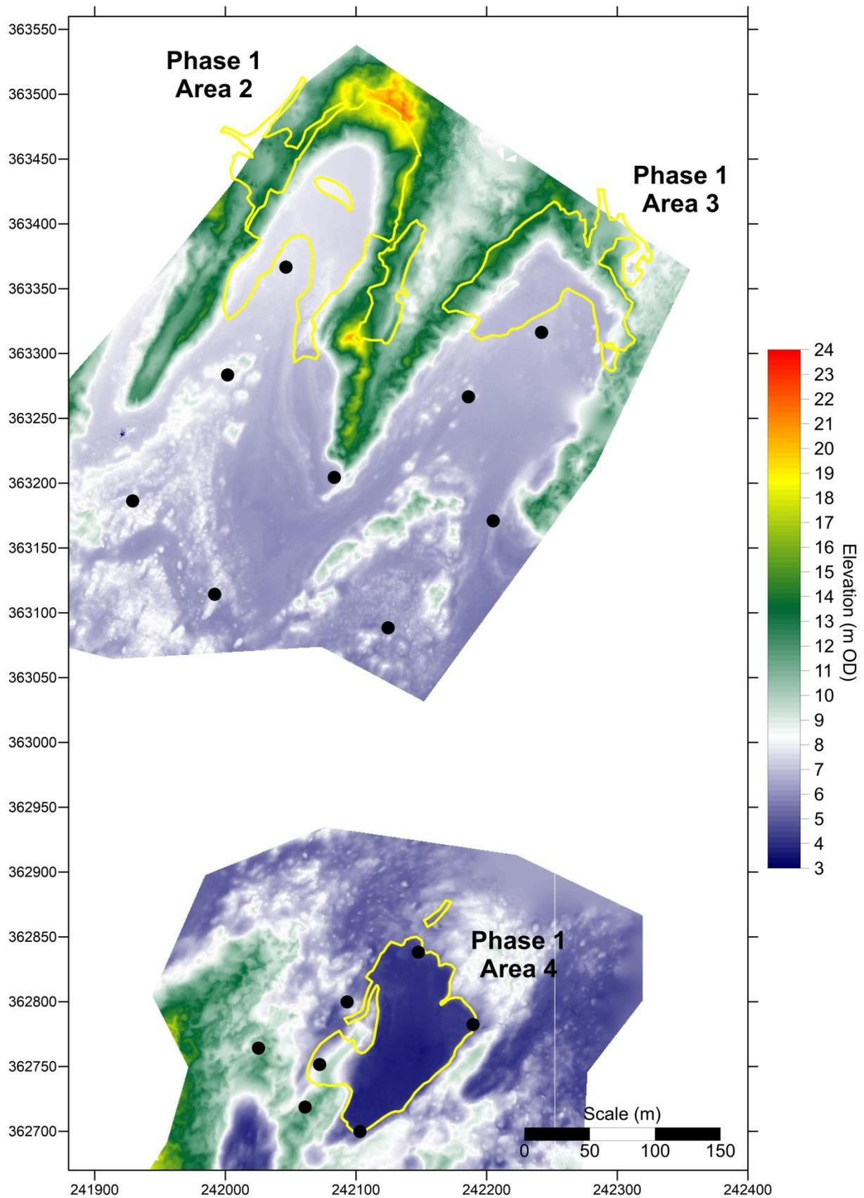
**Figure 56.** DEM of Newborough Warren Phase 1 areas, from a UAV survey in January 2016, after the rejuvenation works. The calibration points used by the survey company to correct the elevations are shown as black dots
