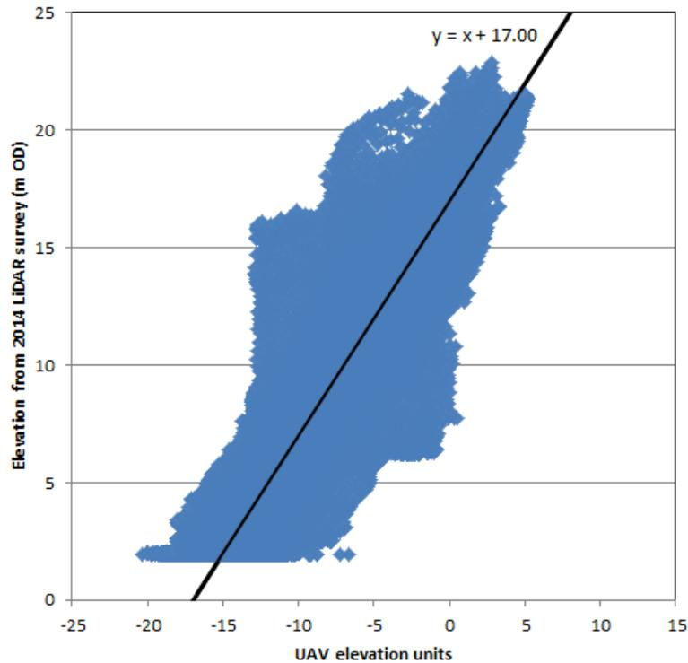
**Figure 16.** Comparison of elevation units measured during 2014 LiDAR survey and 2016 UAV survey, after translation of 3 m to the south and 5 m to the west. A linear trend line shows that an initial correction of +17.0 m is required to adjust elevation units to ODN
