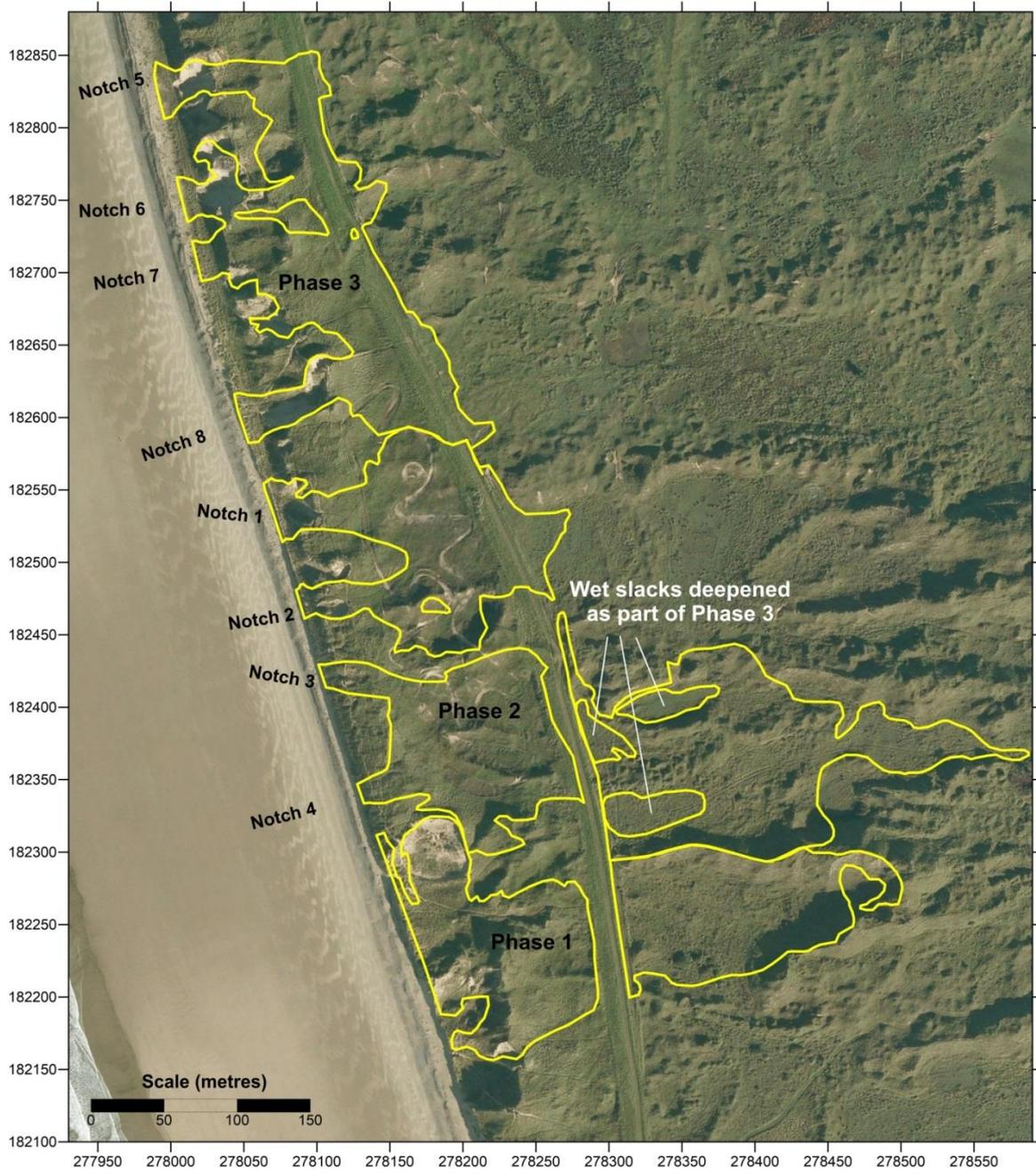
**Figure 4.** Pre-works aerial photograph flown 12 October 2009, showing boundaries of the Phase 1, 2 and 3 rejuvenation trial areas and positions of the major notches
