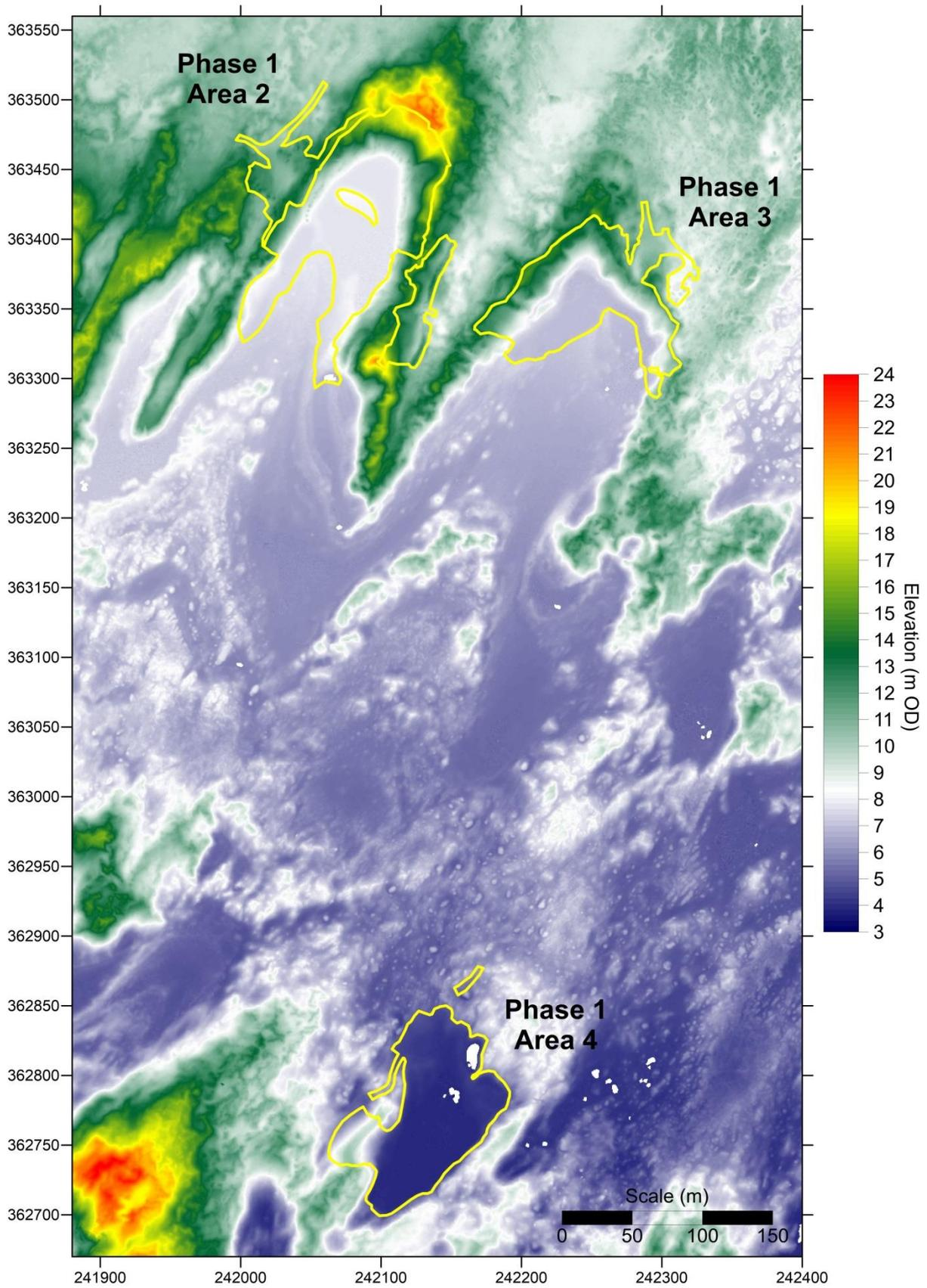
**Figure 54.** Unfiltered DEM of Newborough Warren Phase 1 areas, from an aerial LiDAR survey flown on 9 April 2014, after the rejuvenation works
