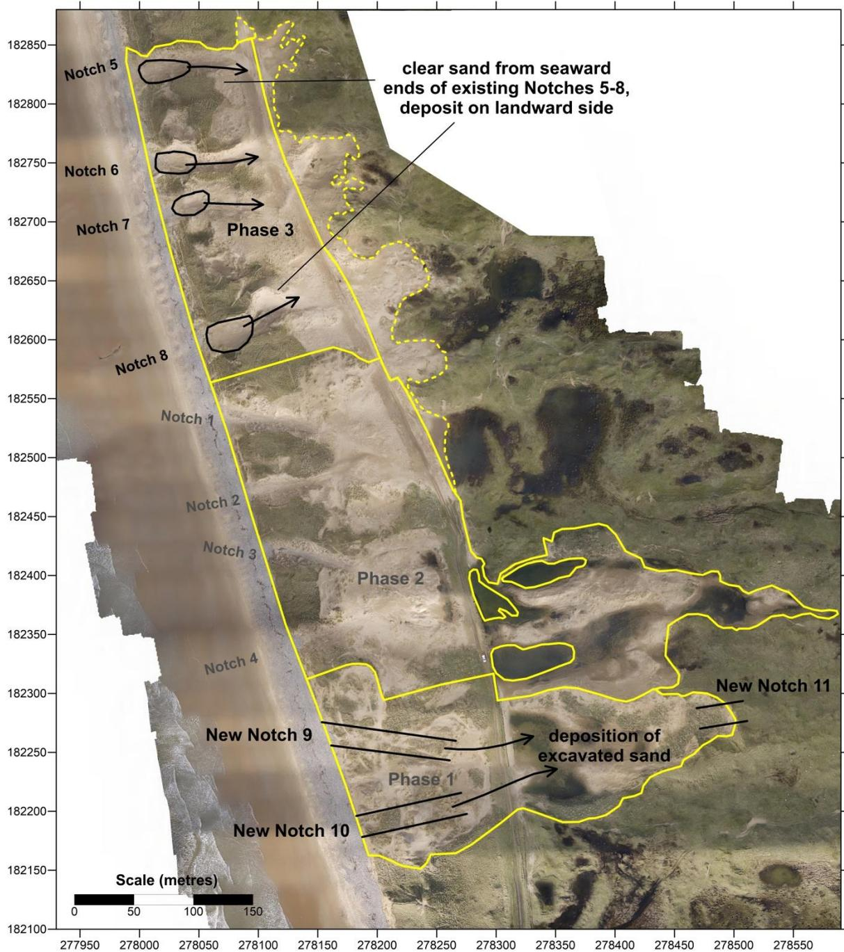
**Figure 91.** Proposals for further intervention works at Kenfig Burrows: (A) creation of two notches through the frontal dunes within the Phase 1 West area, with translocation of sand to the east side of the haul road (Phase 1 East area); (B) creation of a 3 m deep, 10 m wide notch in the crest of the parabolic dune in the Phase 1 East area; (C) removal of sand obstructing the mouth so the Phase 3 notches and deposition on the west side of the haul road behind the notches.
