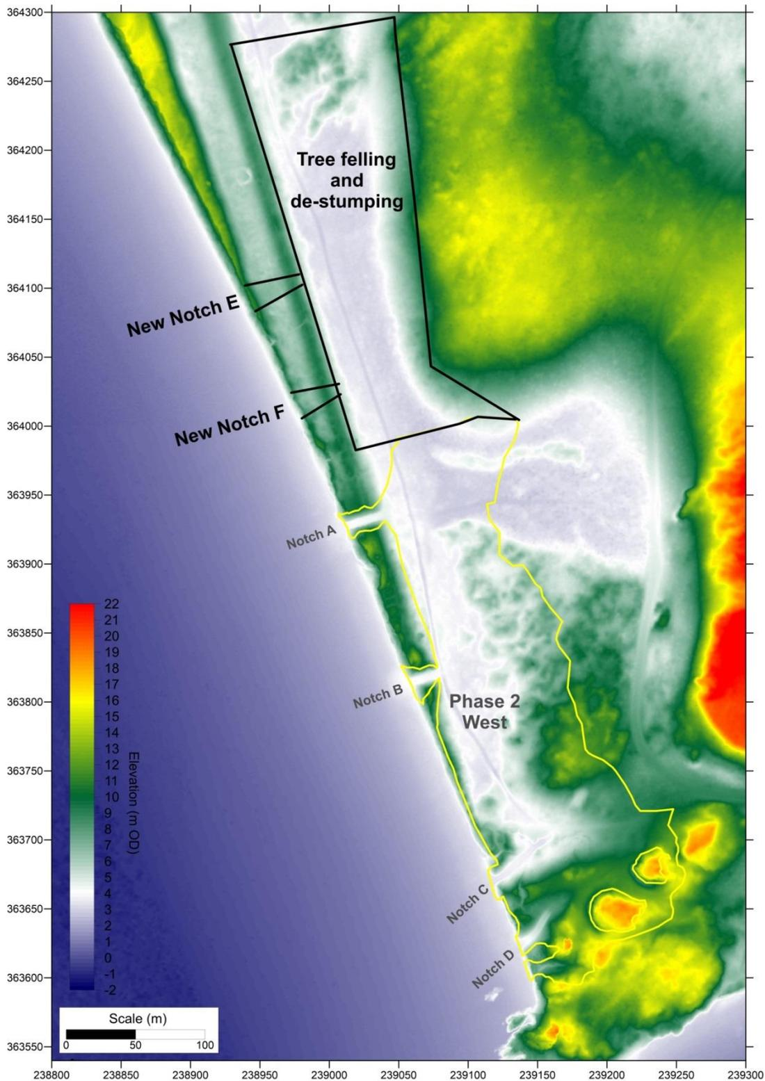
**Figure 94.** Proposals for further intervention works at Newborough Forest (Traeth Penrhos): (A) tree felling and de-stumping in the degraded frontal dune woodland area to the north of the Phase 2 clearance area; (B) creation of two additional notches in the frontal dune to link the beach with the additional forest clearance area, each notch having a trapezoidal plan form and relatively steep seaward gradient to focus wind flow in both the horizontal and vertical dimensions
